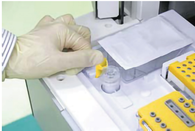
Figure 29. Removing old polymer cartridge.
