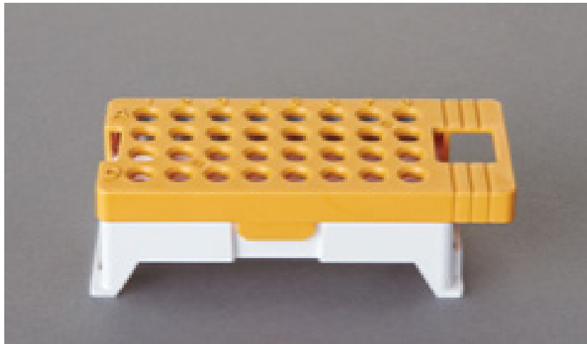
Figure 14. Assembled Spectrum Compact Sample Cartridge.
