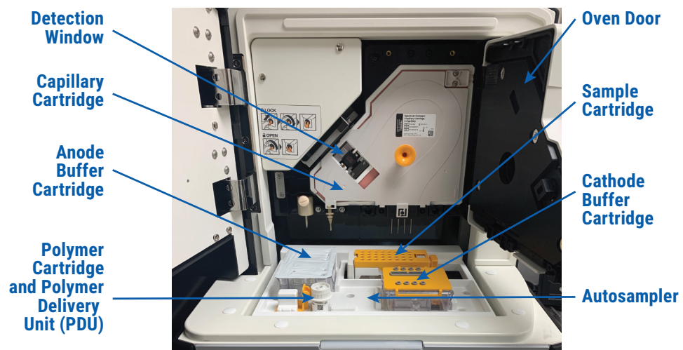
Figure 3. Interior of the Spectrum Compact CE System. The interior of the system provides access to key components. Instructions for maintaining the buffer, polymer and capillary cartridges are provided in Section 3, Managing Consumables.
