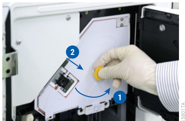
Figure 41. Removing the capillary cartridge.
