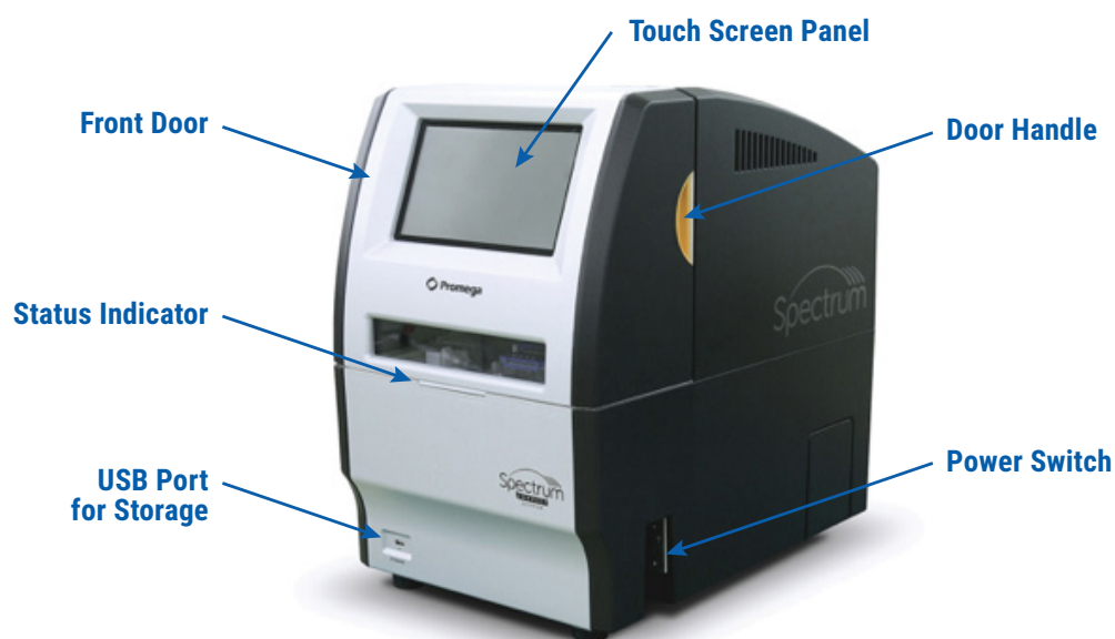
Figure 1. Front of the Spectrum Compact CE System. Front view showing touch screen panel, front door, status indicator and USB port. The power switch and door handle are located on the right side of the instrument.
