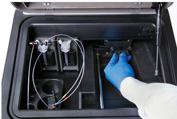
Figure 101. Replace the Aperture.
